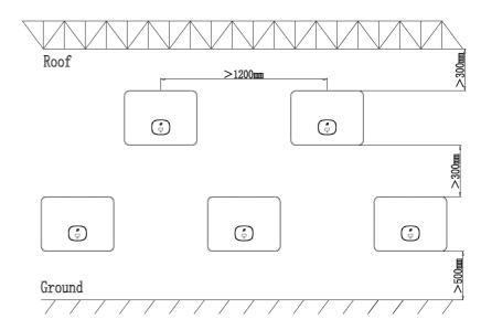
Fig 5.3 Installation dimensions for multiple inverters
