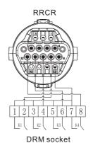
Fig 6.17 Inverter - RRCR Connection
