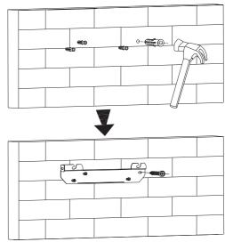
Fig 5.8 Schematic diagram of wall mount installation
