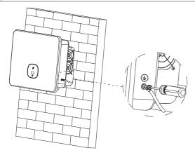
Fig 6.1 Grounding diagram
