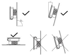
Fig 5.1 Installation diagram
