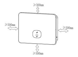
Fig 5.2 Installation dimensions for one inverter
